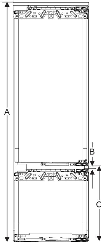
Fig. 68 Clearances for a 2-door cabinet door
